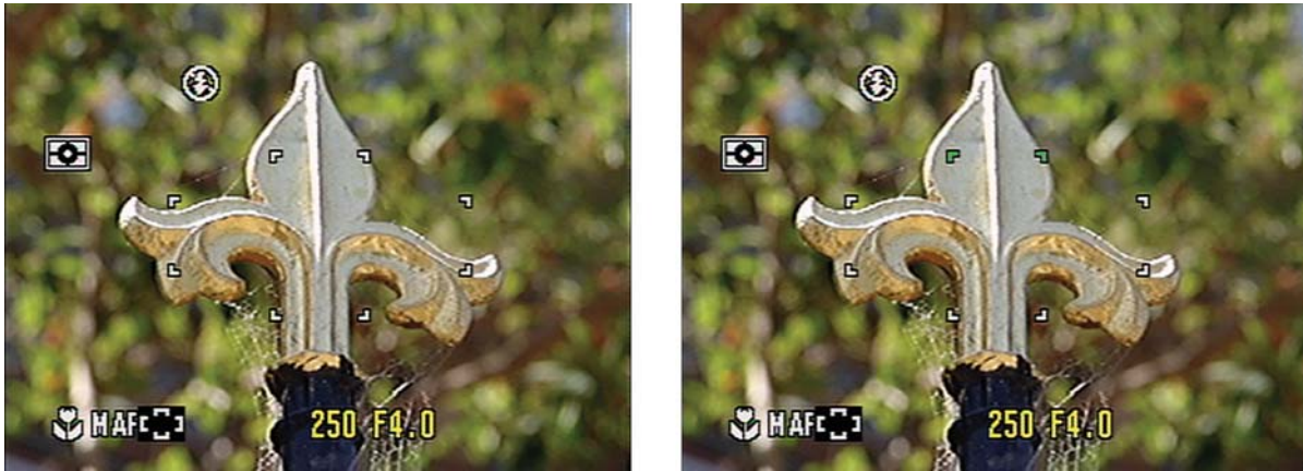
Figure 23.24 Many cameras have multiple focus spots. When you press the shutter button halfway, the camera determines which focus spot is on your subject, automatically focuses the lens to that point, and locks the focus. Here, the camera has selected the upper focus spot.
