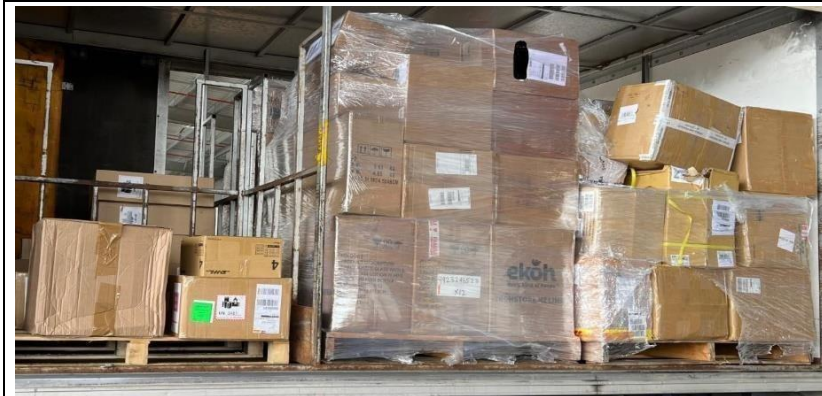
Picture 16.4: Pallets which contain cartons not wrapped to pallets or with loose packages on top of the pallet will be rejected .
