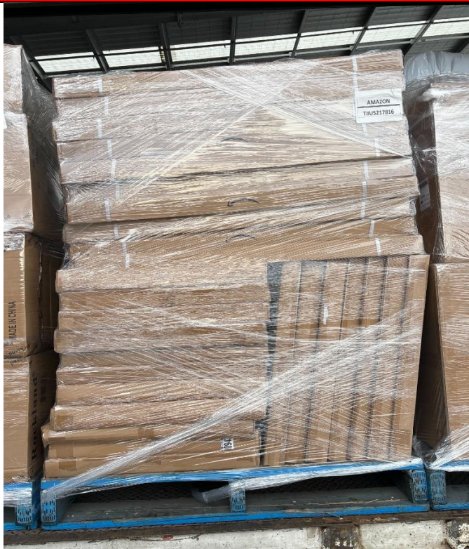
Picture 17.13: Pallets loads not wrapped with enough tension or the loads are not stacked correctly – this pallet load becomes unsafe to be unloaded. This will be rejected .
