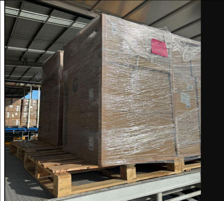
Picture 17.12: The wrapping overlaps with the other pallet. This will be rejected .
