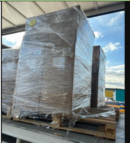
Picture 17.10: The tails are unsecured, and the pallet load is not anchored securely on the pallet bed. This load will be rejected .
