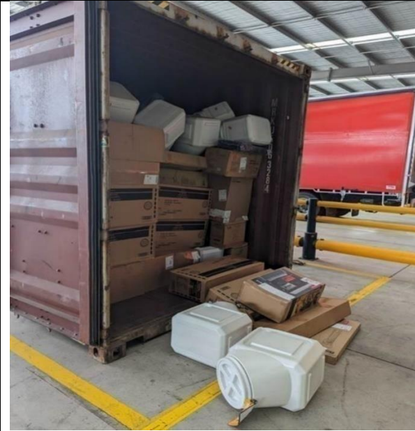
Picture 16.8: Products falling out due to the absence of cargo nets poses a risk of head injuries, and this will be rejected .
