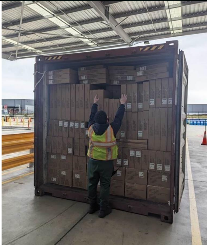
Picture 16.7: Products stacked too high without 8 cm of clearance at the top of the container – this will be rejected .
