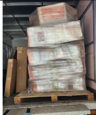
Picture 16.5: Poorly stacked pallets or products not safely wrapped to the pallets will be rejected .
