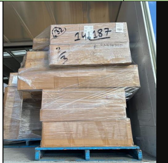
Picture 17.11: The wrapping is not anchored to the top 30-50% of the pallet, and the top load is overhanging. This will create unstable pallet movement. This pallet will be rejected .
