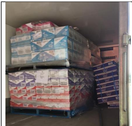
Picture 16.1: double stacked pallets or single stacked pallets without the required 15cm clearance at the top of the truck, with products not wrapped to the bottom pallet or with fallen products next to pallets (which risk being damaged when pallets are removed) will be rejected .
