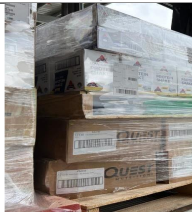
Picture 16.3: Pallets which are too close together, which risk one pallet being damaged whilst unloading, where products may become dislodged or which are no longer wrapped to the pallet will be rejected .
