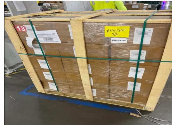
Picture 16.6: Freight packaged this way would be rejected as we need to use tools to force open the package and may damage the inventory
