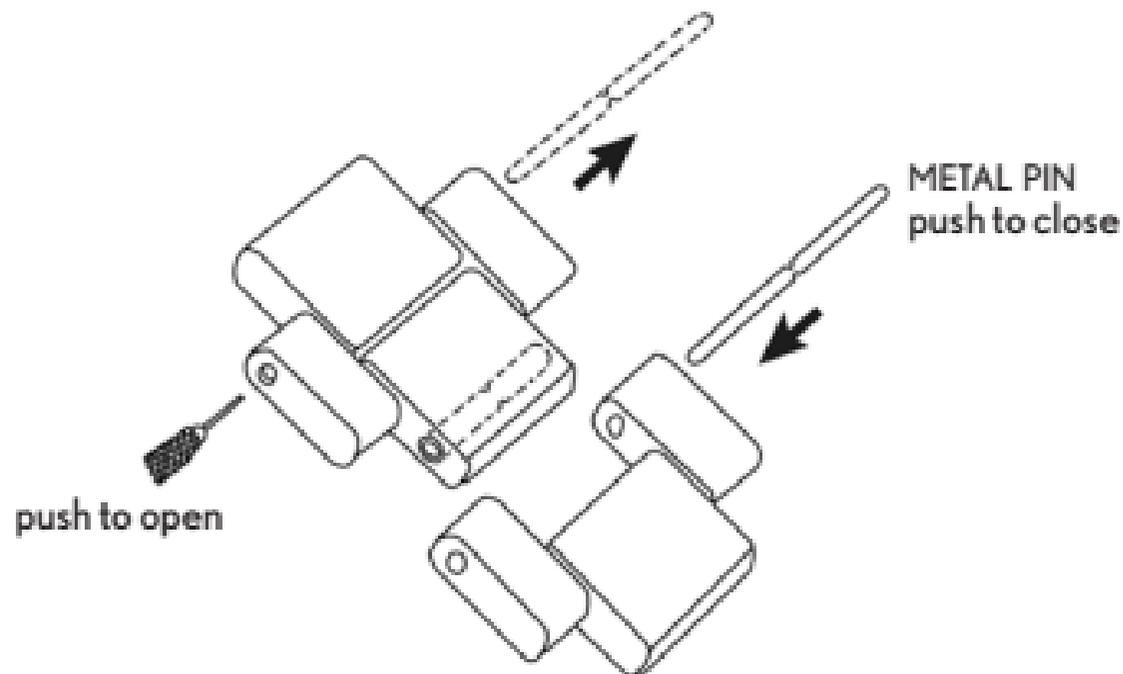
In order to adjust links for this watch construction, you must switch the pin on the tool kit to the longest pin (approximately 10mm long) found under the tool kit. Then use the pin remover tool to push out the pins from either side of the links. After the desired links are removed, simply follow these steps in reverse to re-assemble the bracelet.
