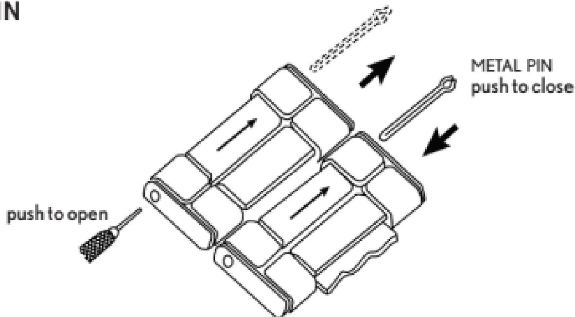
Turn over the watch to look for arrows on the underside of the links, showing you which way you need to push the pin out of the link. Use a pin remover tool to push out the “hair clip pin” from the hole located on the side of the link. After the links are removed, simply follow these steps in reverse to re-assemble the bracelet.
