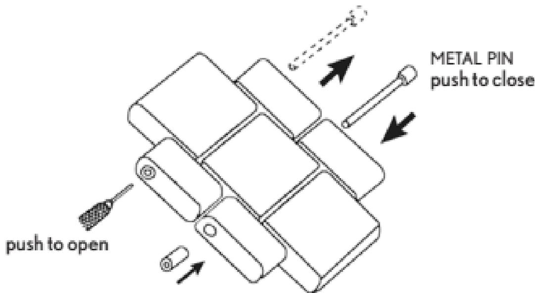
Check the side edge of the watch link, to determine which side of the link is "**A**" or "**B**". Take a pin remover tool and push out the pin from the hole located on side "**B**". After the desired links are removed, simply follow these steps in reverse to re-assemble the bracelet.
