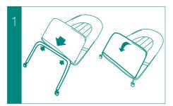
Slide the footrest frame inside the fabric cover as shown.
