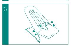
Push the ends of the leg wires through the plastic mouldings on the legrest frame.
