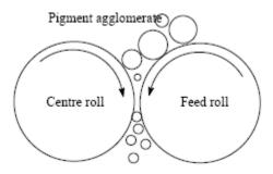
Figure 1 - Pigment Particles enterting a three roll mill
