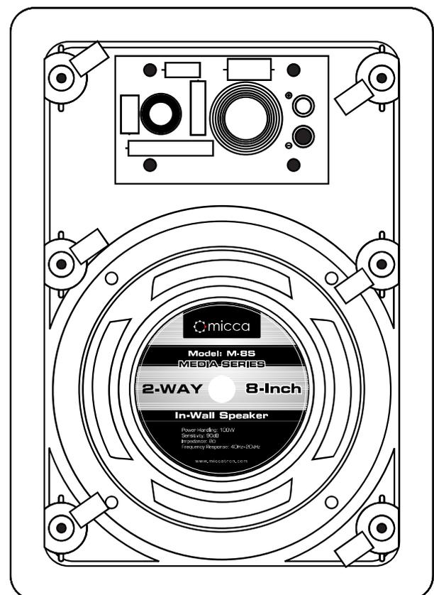
Place the speaker into the wall cutout. One at a time, loosen each of the six screws until the tabs can turn freely. Next tighten each screw clockwise until the tabs press firmly against the inner wall surface. The speaker need only be properly aligned and held securely to the wall – do not over tighten to break the tabs or damage the wall.
