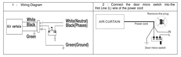
The air curtain should be installed indoor, please follow the below diagrams for the recommended installation.
