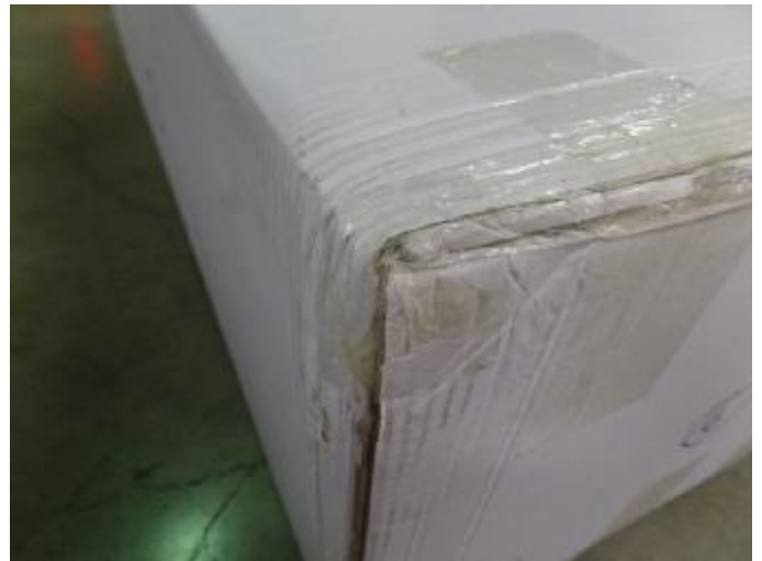
Compression Fatigue – Corner 3-4-6
