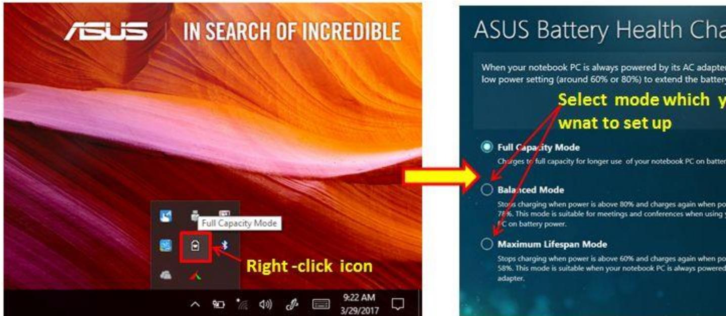
A. **Full Capacity Mode**(Yellow color): Battery is charged to its full capacity for longer use on battery power.
