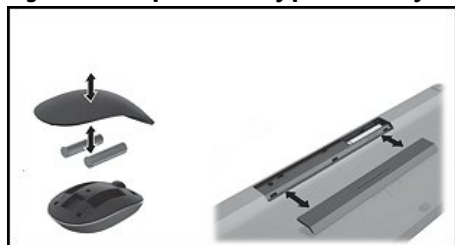
Figure 6: Example of battery placement - yours might vary
