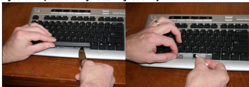
Figure 7: Example of removing and cleaning a stuck key
