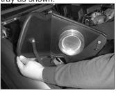
18. Install the heat shield assembly.
