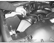
30. Install the Air filter element and secure with hose clamp.
