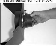
10. Assemble the mass air sensor, heat shield and adapter using the gasket and hardware provided.
