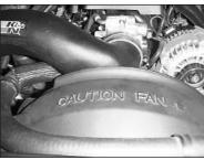
29. Due to production tolerances it may be necessary to mark the fan shroud as indicated, remove the intake tube and trim the fan shroud.
