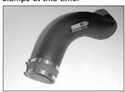
23. Install the 3.75"ID silicone hose (08631) onto the intake tube.Note: Do not tighten the hose clamps at this time.
