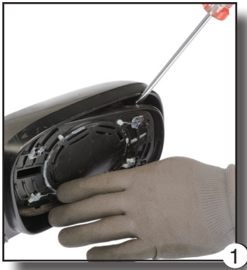
Fig. 1. Removing the broken mirror glass assembly from the current housing.
