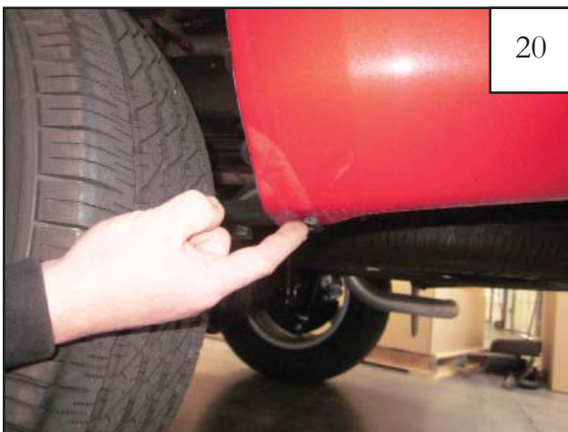
NOTE: If the lower rear wheel well does not contain a plastic grommet, insert supplied Grommet (GR1-0001) into the factory hole as shown.
