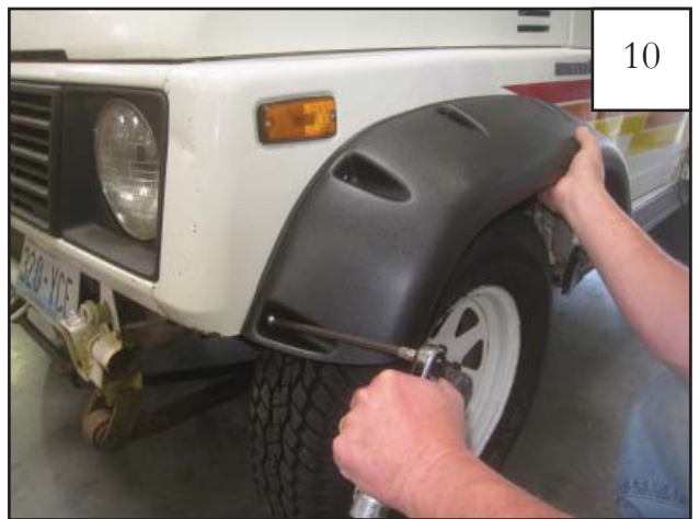
Hold the flare to the fender, lining screws up with 3/16" drilled holes and start screws into sheet metal. Once all screws are started, tighten to 2 ft•lb of torque.
