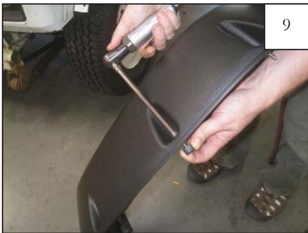
At each flare pocket, insert a #45 Torx screw and run it into a rubber spacer until snug with the flare plastic. Use a 5/16" socket and 6" extension to prevent marring flare plastic. Wrap a layer of masking tape around torx bit to help it stay in the socket.
