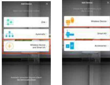
5) Make sure that your NVR is powered on and connected to your WiFi router. Connect your NVR to your WiFi router using an Ethernet cable (provided). Please make sure that your smartphone is connected to the same WiFi network that your NVR is connected to.
