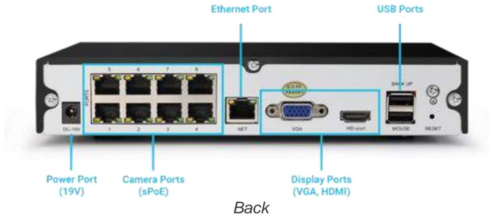
This NVR is specifically designed to support wired surveillance cameras. The cameras use one custom sPoE cable to provide both power and video from the NVR to each camera for easier installation. When installing the hard drive, you will need to loosen all case screws and remove the top panel.
