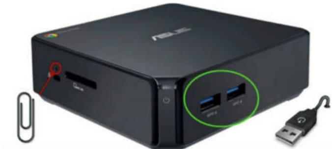
3. Press down the recovery button with the paperclip while turning on the Chromebox
