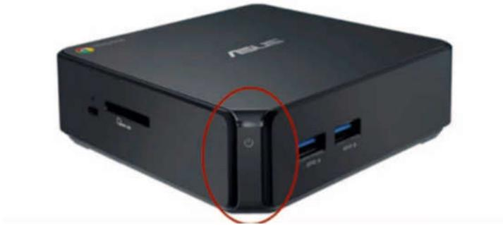
2. Connect a USB Keyboard to the front of the Chromebox, and put a paperclip into the recovery button hole:
