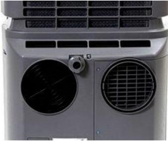
Operationally, a dual hose portable air conditioner has two main advantages over a single hose unit. A dual hose portable air conditioner will cool a room faster and will help minimize negative air pressure situation in the room. If the outside temperature is much higher or more humid than the room, the intake hose can be covered with the included cover and it will function like a single hose unit.
