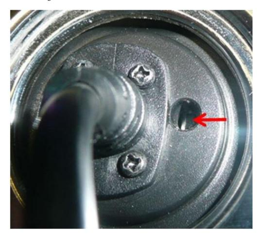
3. Press (and hold pressed) this button with a small screwdriver (you must hear a small "click" noise)
