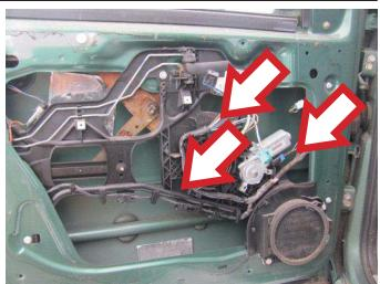
**STEP 8a:** Attach the electrical connector to the window lift motor.
