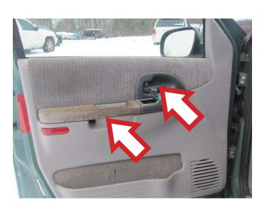
**STEP 2:** Remove the master switch assembly by using either your plastic pry tool or a flat-blade screwdriver.
