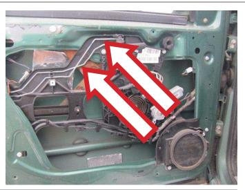
**STEP 8:** Attach the door wiring harness assembly onto the window regulator module assembly.
