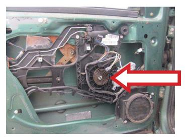
**STEP 6:** Disconnect the electrical connector at the window lift motor.
