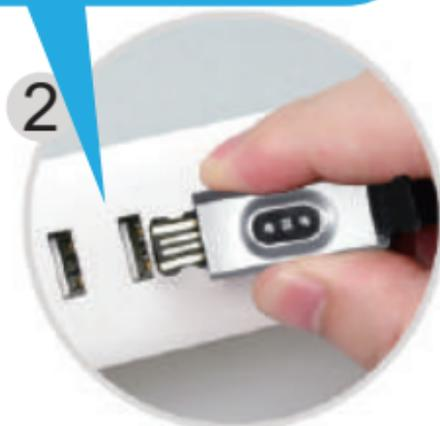
The red indicator is on when the device is properly charged. If not, check the direction of the device's charging plug and move to the correct direction, as shown below.
