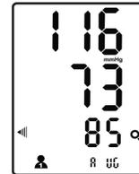
2. Press MEM button or SET button to rotate the records. Up to 60 records will be stored under each user ID.
