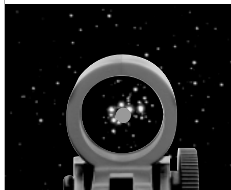
Figure 7. EZ Finder II superimposes a tiny red dot on the sky, showing right where the telescope is pointed.
