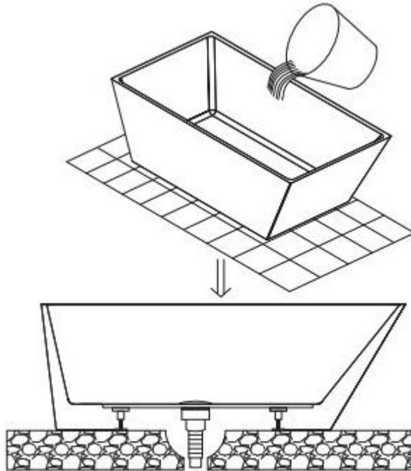
**2-5. Apply a thick layer of silicon sealant around the bath outline allow it set 24 hours. This installation guide, the installation of waste connection should be only suitably by qualified person.**
