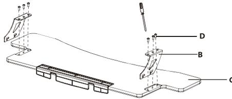
Screw assembled keyboard tray and hinges (B) onto adjustable desktop.
