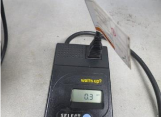
Plug the cord into socket. Here using a watt meter.
