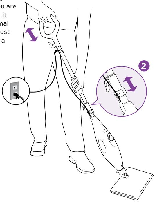
**2** Pump the handle a few times in a downward motion. This pumping action will release steam as you mop and allows you to customize the amount of steam you want. Begin mopping with a forward and backward motion. The natural motion of mopping will produce steam.
