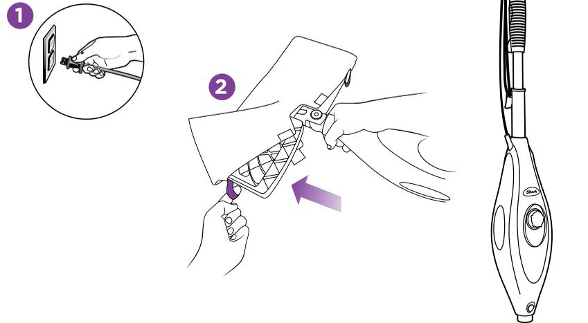
2 Remove the micro-fiber cleaning pocket by releasing the quick fasteners and using the lavender loop on the side of the pocket, avoiding contact with the hot pocket or dirt. Then empty the water tank.
