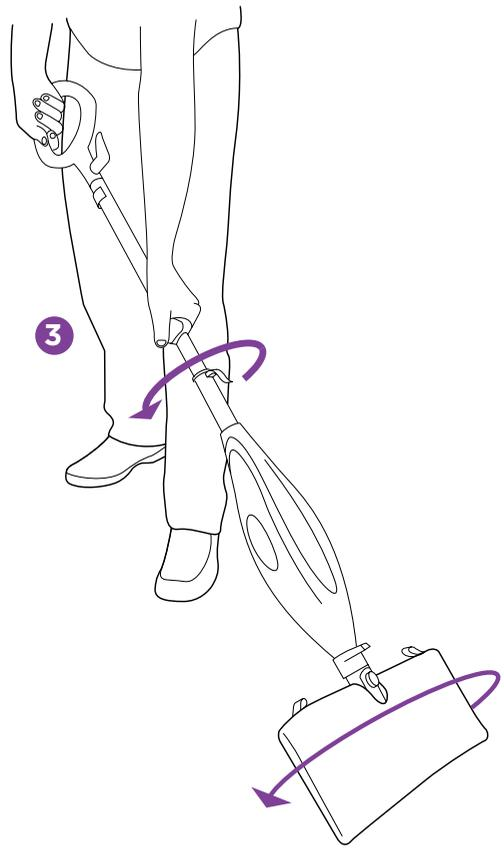
**3** When one side of the micro-fiber pocket gets dirty, just flip the mop head and you can quickly start using the other side. Dirt can't hide on either side.
