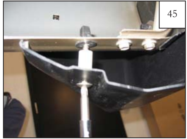
At bottom rear of flare, install a supplied Screw (SW1-0034) and a Spacer (SP1-0008).
