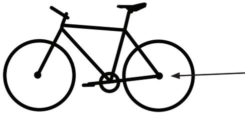
The dropouts are located here. They are the two slots that the axle connects to. They hold the rear wheel in place.
