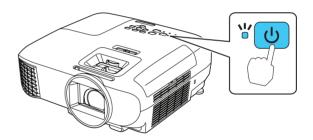
**Note:** To shut down the projector, press the opower button twice.
