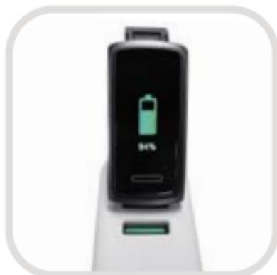
If the tracker does not vibrate, remove the tracker, flip it upside-down and reinsert it into the charging port.
