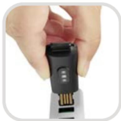
When the tracker shows a low battery indication, connect the tracker to a USB charging adaptor or a port with 5V-500mA. If the tracker is installed correctly, the tracker will vibrate.
