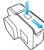
2. Insert a microSD card with the label facing the battery (microSD card is not required for charging).
