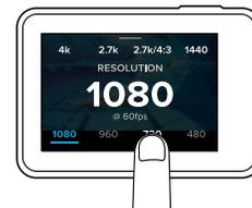
If you select a video resolution (RES) that does not support the frames per second (FPS) setting that is selected, a message appears that instructs you to tap the touch display to automatically move to the FPS setting and select a different value. A similar message appears if you select an FPS that is not supported by the selected resolution.
