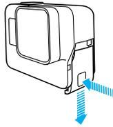
5. Connect the camera to a computer or other USB charging adapter using the included USB-C cable.
