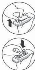
**NOTE:** Do not use rechargeable batteries. Make sure that both batteries are new.
