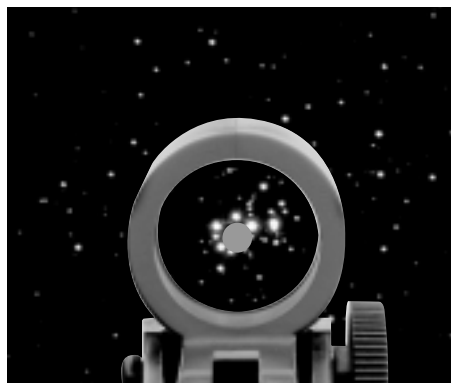
Figure 6. EZ Finder II superimposes a tiny red dot on the sky, showing right where the telescope is pointed.
