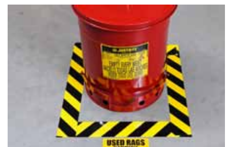
Hazard area (black/yellow)
