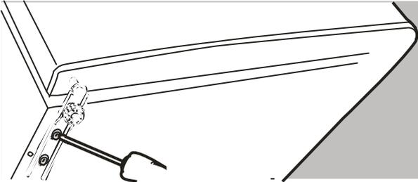
7. Check that the door is aligned horizontally and vertically and that the seals are closed on all sides before finally tightening the bottom hinge. Readjust the leveling feet.
