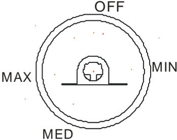
When using the refrigerator-freezer for the first time or after defrosting, turn the temperature control to set "MAX" for at least two hours before introducing the food to be stored. All frozen food products you purchase should be placed in the freezer compartment as soon as possible to avoid the frozen food from defrosting.
