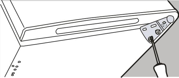
6. Screw the bottom hinge into place on the new side. Replace the foot on the other side.
