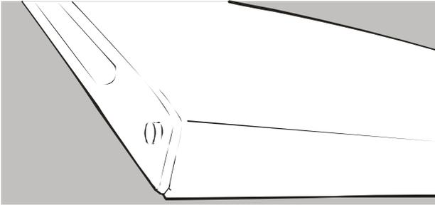
4. Remove the plastic cover from door hinge first. Then unscrew the two screws from top bracket and replace on the other side.
