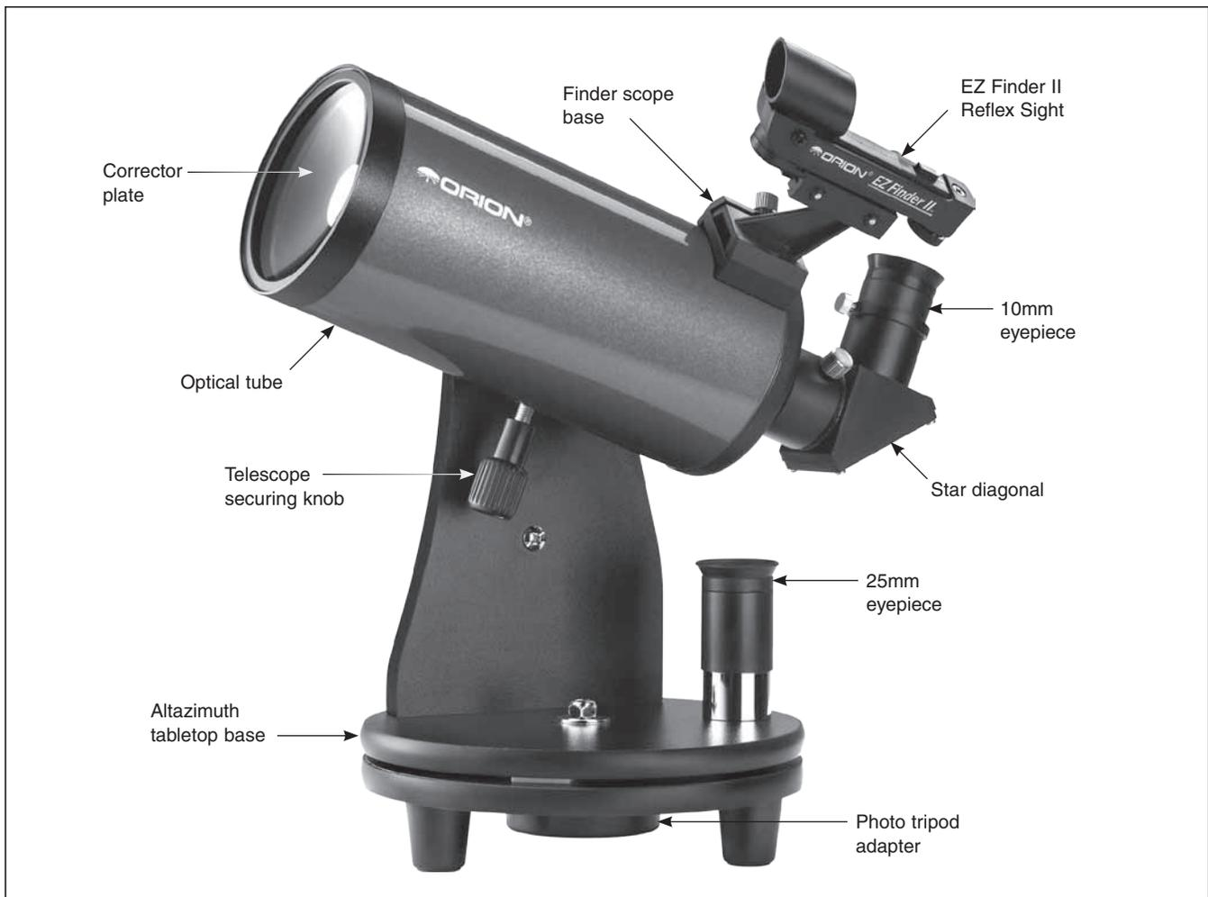
**Figure 1b:** The StarMax 90 TableTop Telescope
