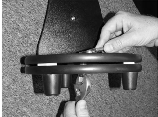
**Figure 11:** Making optional adjustments to the azimuth tension
