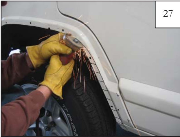
Use a cut off saw to cut the front fender along marked line. Do not cut any sheet metal past where the horizontal lines were marked in step 25.
