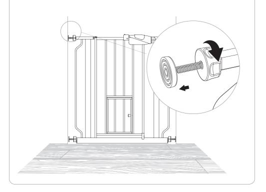
**NOTE:** It may be necessary to hold the *threaded spindle rods* or *rubber feet* while rotating the *adjustment wheels* to ensure the entire unit does not rotate.
