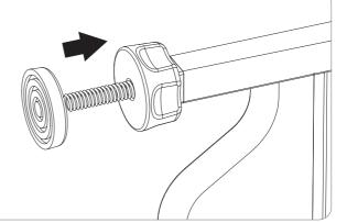
**NOTE:** The ends of the gate frame are not threaded. The *threaded spindle rods* should slide into the end of the frame tubes without any resistance.
