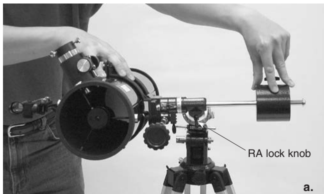
Figure 4. Proper usage of the equatorial mount requires the telescope tube to be balanced on both the R.A. and Dec. axes. (a) With the R.A. lock knob released, slide the counterweight along the counterweight shaft until it just counterbalances the tube. When you let go with both hands, the tube should not drift up or down. (b) With the Dec. lock knob released, loosen the tube ring lock clamps a few turns and slide the telescope forward or back in the tube rings. When the tube is balanced about the Dec. axis, it will not move when you let go.
