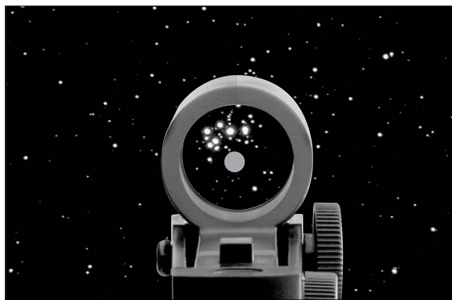
Figure 7. The EZ Finder II superimposes a small red dot (it's not a laser!) on a non-magnified field of view, which helps to center an object in the telescope's field of view.
