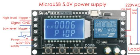
Weak current control strong current wiring diagram
