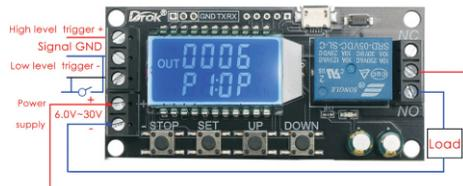
Wiring diagram for sharing one power supply
