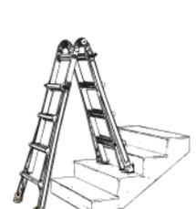
Start from the small A-frame position; lengthen the down side of the ladder to the desired height. Ensure the ladder rungs are level before using.
