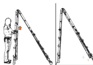
From the tall A-frame position reduce the height on one side of the ladder by one foot. Make sure the ladder is on a flat level surface and the short side of the ladder is against a secure wall.
