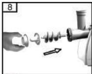
6. Then fasten the tightening ring around the kibbe tube, turning it clockwise to secure.
