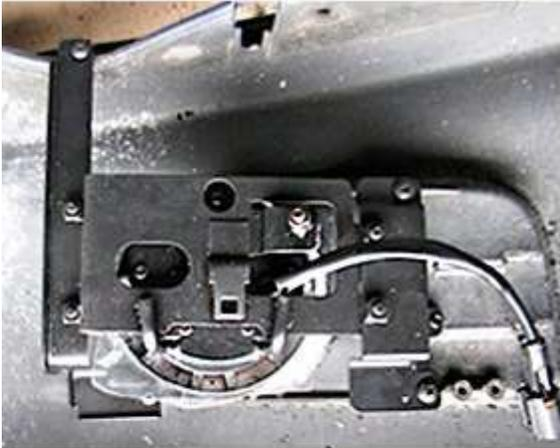
Here, a fog light mounting bracket for a vehicle-specific kit is shown after being installed.
