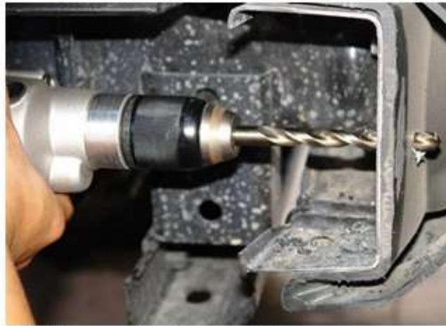
Drill bits specified for metal are recommended when drilling into any bumper or vehicle frame sections during fog light installation.
