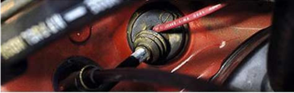
Most vehicles have a hole in the firewall pre-drilled at the factory for the purpose of running wires from under the hood to the interior.
