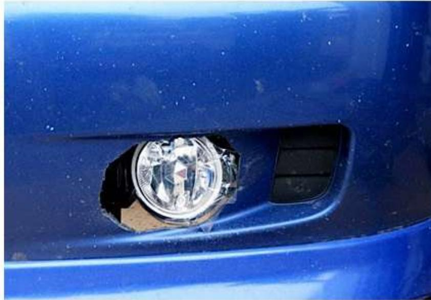
Here, the outside of the bumper cover in the previous photo is shown. It's always a good idea to use the fog light you'll be installing as a template. After drawing a line around it on the back side of the bumper cover, follow the lines as closely as possible when cutting.
