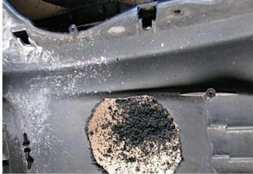
This picture shows the inside of a front bumper that was not originally equipped with fog lights, but has a pre-determined area for mounting them.
