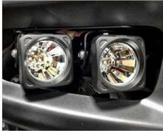
This picture shows just one example of how a universal aftermarket fog light bracket and lights can be installed after custom drilling.
