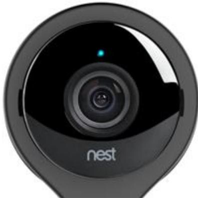
**Plug the other end of the cable** into a USB port on your computer. The light on the front of your Nest Cam will glow blue (yellow on Dropcam), telling you that the camera is booting up. After a moment, the light will begin blinking.
