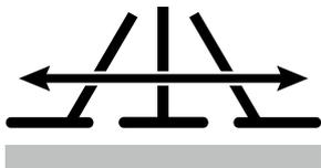
**SWEEP LEVEL** Keep the coil 1–2 inches (2–3 cm) above and parallel to the ground at all times.
