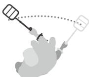
**SPEED** Sweep the coil over the ground in a side-to-side motion, an average sweep speed is 1–2 seconds from left to right.
