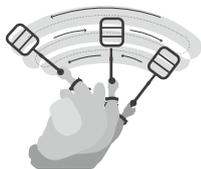
**OVERLAP SWEEP** Slightly overlap the previous sweep to ensure full ground coverage.
