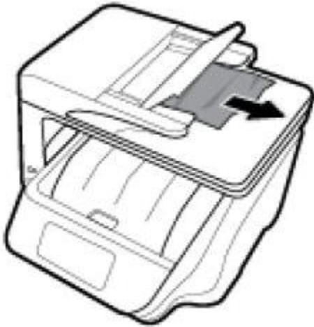
Figure : Removing jammed paper from under the ADF tray
