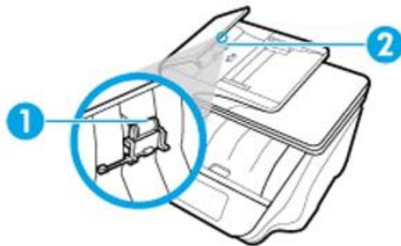
Figure : Cleaning the rollers and separator pad
