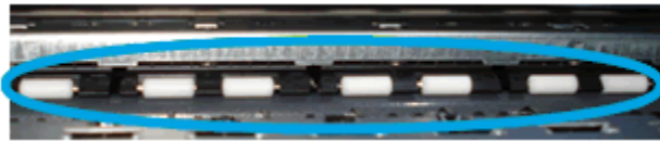
Figure : Clean the rollers in the cartridge access area
