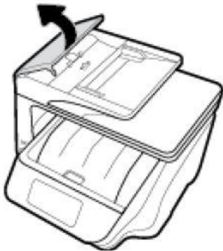
Figure : Lifting the ADF cover
