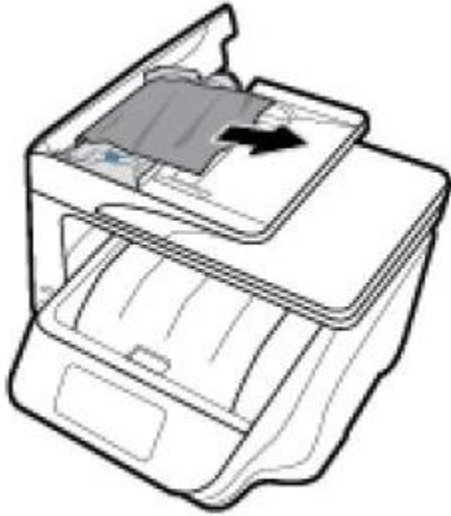
Figure : Removing jammed paper from the rollers
