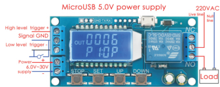
Weak current control strong current wiring diagram
