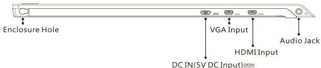
Fig.: On-Lap 2501 Series input/output ports
