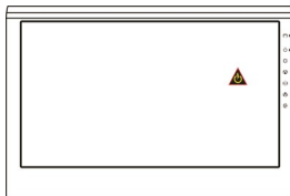
Fig.: Low voltage warning shown at upper right corner on screen.
