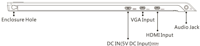
Fig.: On-Lap 2501 Series input/output ports
