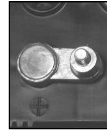
POSITIVE POST HAS LARGER DIAMETER
