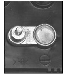
NEGATIVE POST HAS SMALLER DIAMETER
