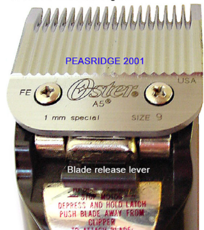
OSTER GOLDEN A5 CLIPPER Fig 1 Blade release lever diagram
