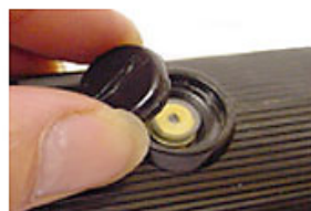
5. Replace carbon brush and brass cap
